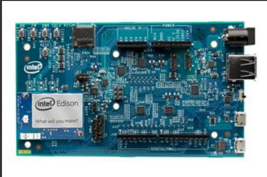
An Intel Edison kit including a full size Arduino Uno with power in and USB ports.
