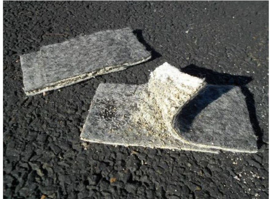
(b) Seam produced with hot air device
