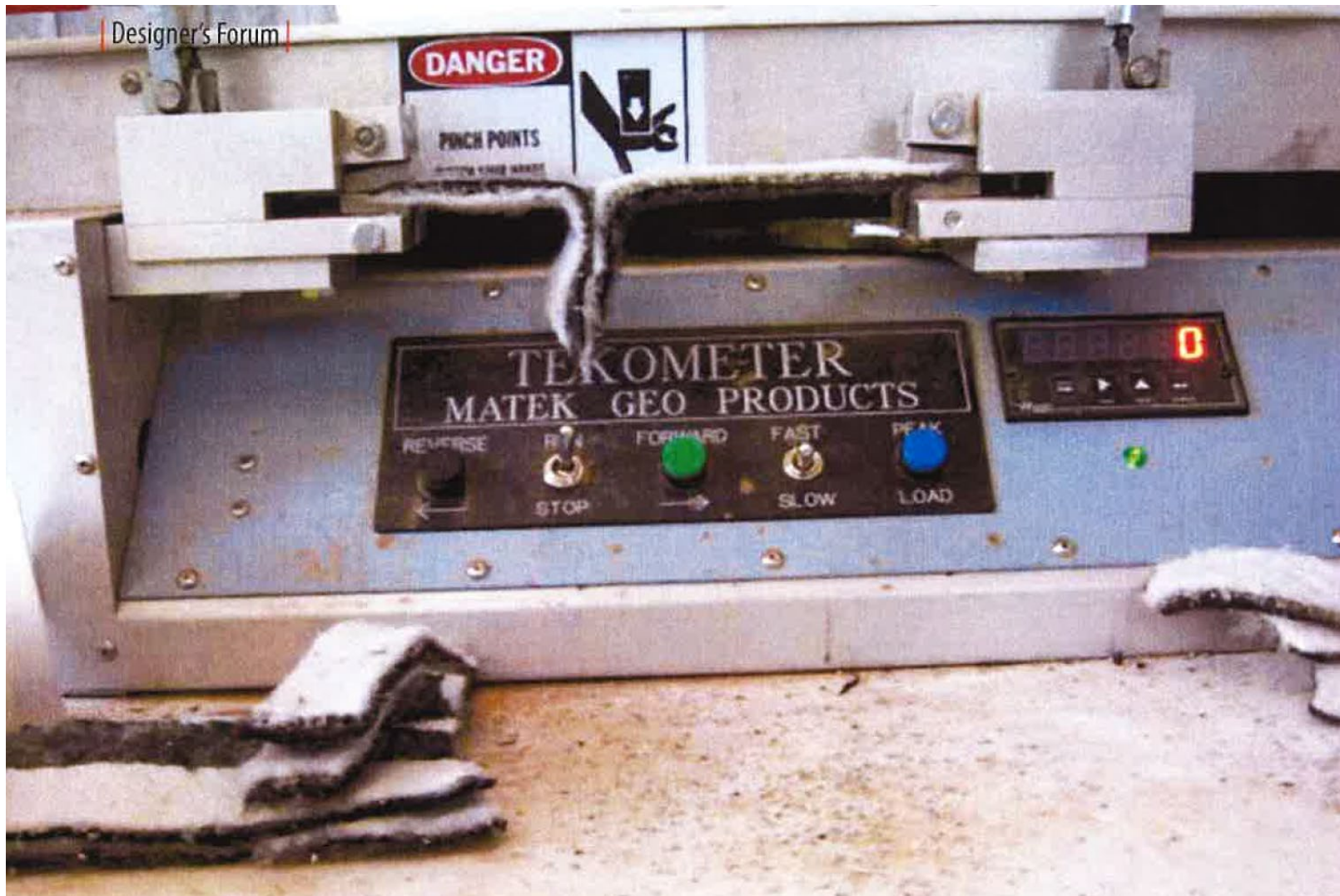
Field destructive testing of the heat bonded seam of adjacent/overlapped GCL panels to form a strong bond. Source: Geosynthetics Feb/Mar 2009
