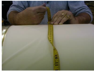
Figure 3: Incorrect Measurement because tape is twisted.
