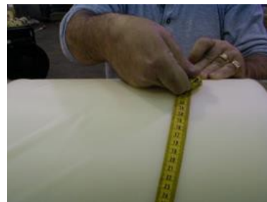
Figure 4: Incorrect Measurement because tape is not parallel to roll edge.
