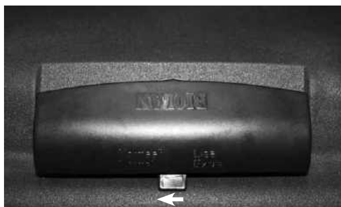
Fig. 4 Air outlet valve in the normal position
