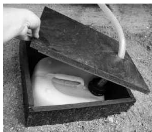
Fig. 3 Tank for collecting seep liquid
