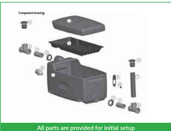
Greywater flows in, cleaned water flows from the base
