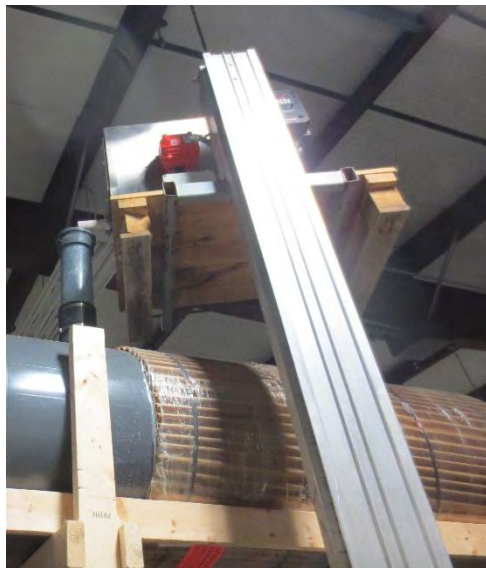
Figure 7 Influent Feed Port for TSS Removal Efficiency Testing
