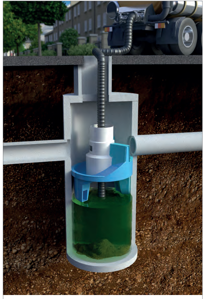
Fig.4 Floatables are removed with a vactor hose
