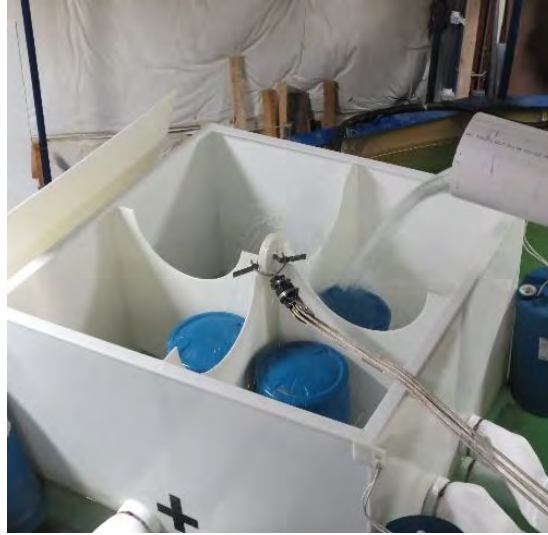
Figure 6 Effluent Sampling Location Situated above the Filter Box
