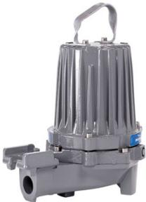
The Flygt M 3000 grinder pumps are high-performing submersible, centrifugal pumps with axial cutters. Excellent for pumping wastewater in residential, commercial and agricultural applications. These grinder pumps reduce waste content to fine slurry, pumped through small-diameter pipes.
