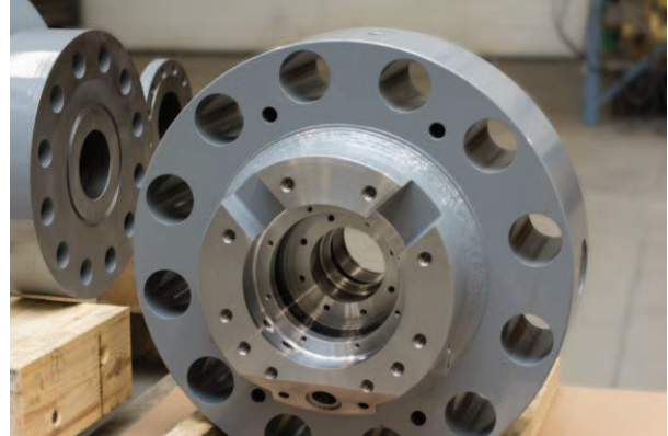
Cast WCB Suction Side Outer End-Head Welded onto forged A105 Inner End-Head
