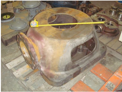
Worn Discharge Head
