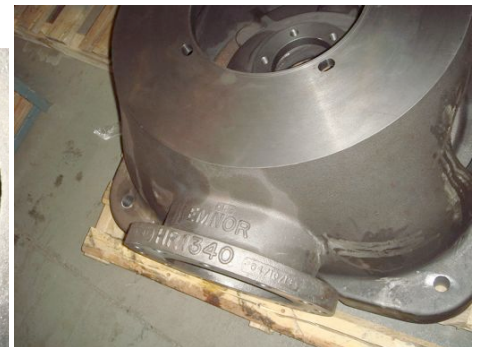
New Discharge Head
