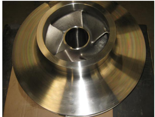
New Double Suction Impeller
