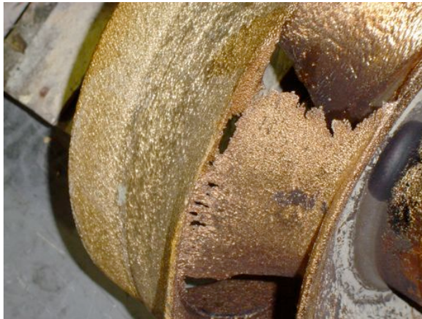
Wear at Outside Diameter
