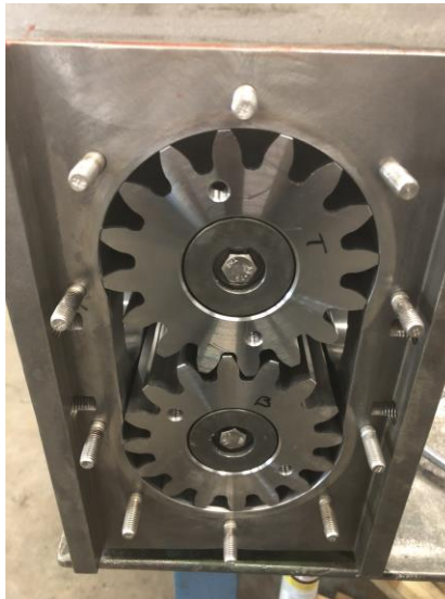
New Gears Installed
