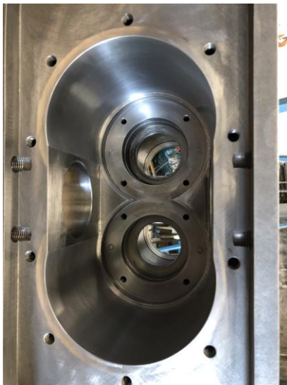
Sleeves Welded Into Housing
