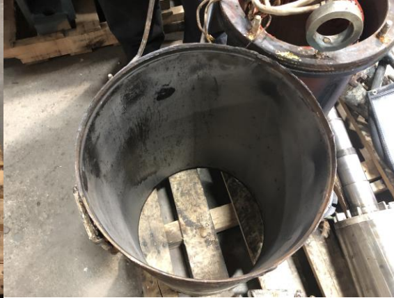
Damaged Cooling Jacket
