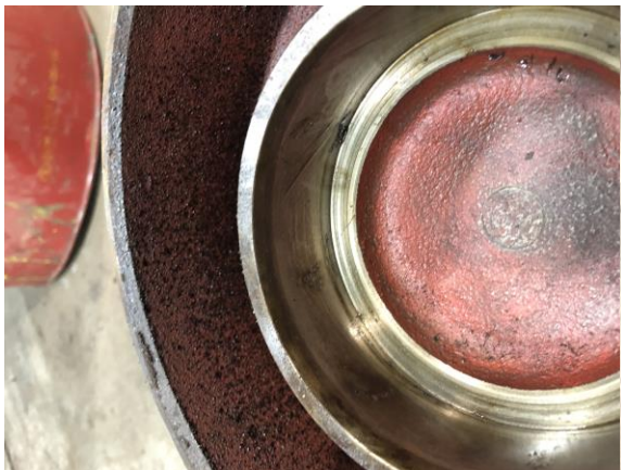
Damaged Bearing Housing Bore
