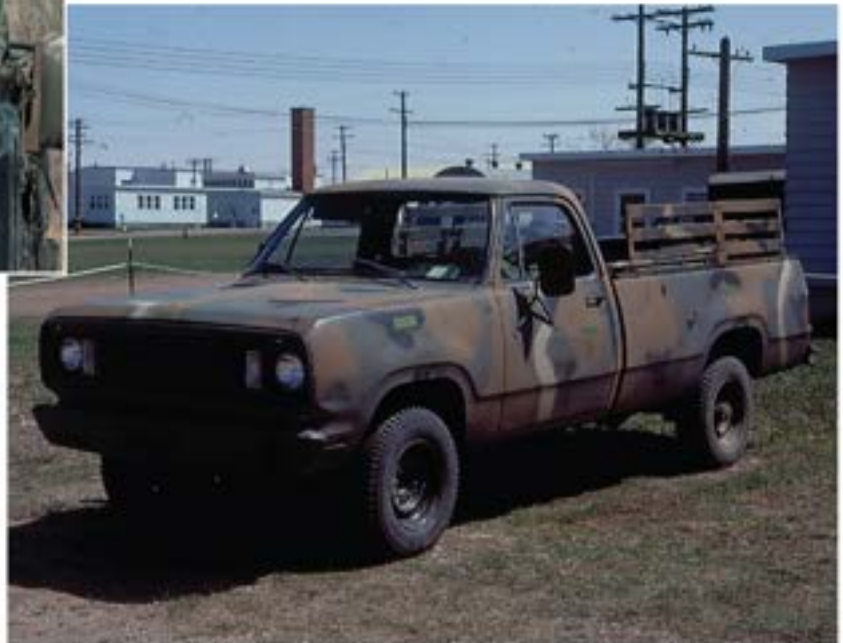
Commercial off-the-shelf vehicles employed by U.S. military involved using existing, commercially available vehicles (sometimes with modifications) to replace or augment more expensive M-series vehicles. This MERDC Verdant Summer camouflaged M880 5/4-ton truck photographed during RV83 was based on the Dodge D250 chassis that featured a 318 cubic inch, V8 engine, a 727 automatic transmission, and full-time 4x4. W.E. Storey Collection
