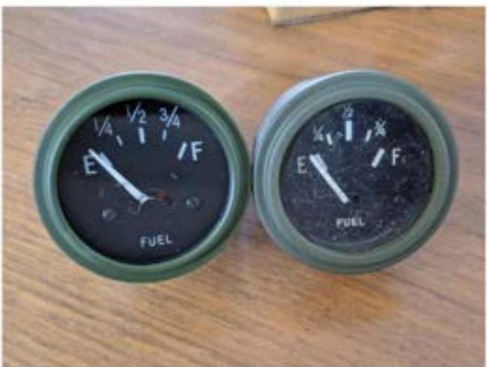
Reproduction fuel gauges (left) are inexpensive and prevent headaches that occur when retaining original gauges (right).
