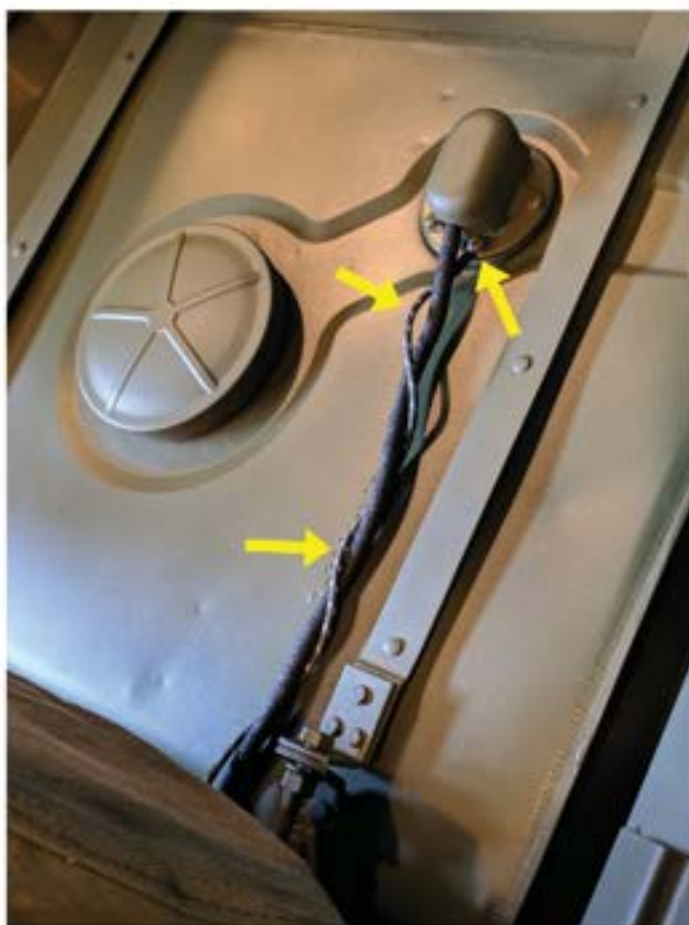
A good ground on the fuel sender is imperative for the fuel gauge to work. A modern solution is to add a second wire going from one of the screws that mount the sender to the tank and connect the wire directly to the body tub.
