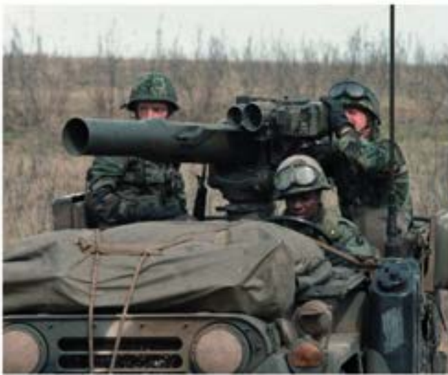
Commercial off-the-shelf vehicles employed by U.S. military involved using existing, commercially available vehicles (sometimes with modifications) to replace or augment more expensive M-series vehicles. This MERDC Verdant Summer camouflaged M880 5/4-ton truck photographed during RV83 was based on the Dodge D250 chassis that featured a 318 cubic inch, V8 engine, a 727 automatic transmission, and full-time 4x4. W.E. Storey Collection
