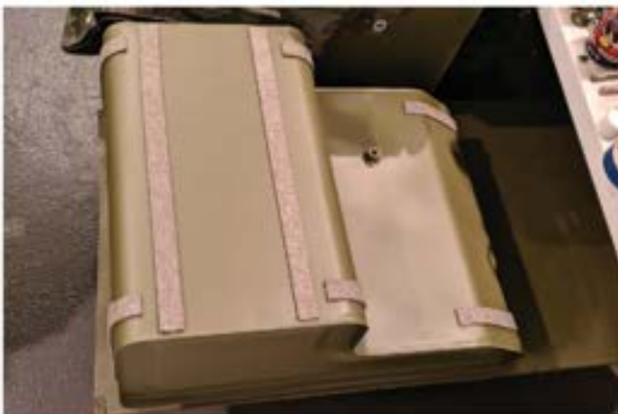
Originally, strips of tar-like coated, cotton duck webbing provided anti-squeak dampening on the bottom of the tank. Today's reproductions use felt.
