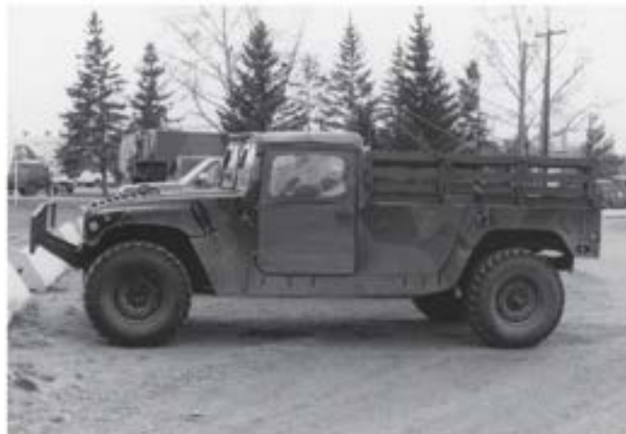
This High Mobility Multipurpose Wheeled Vehicle (HMMWV) M998 cargo carrier without winch had an impressive front early model brush guard mounted on it during RV89. W.E. Storey Collection
