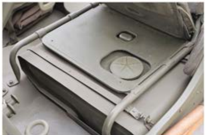
To refill fuel on a WWII jeep, one must simply exit the vehicle, lift the driver's seat cushion, and unscrew the cap.
