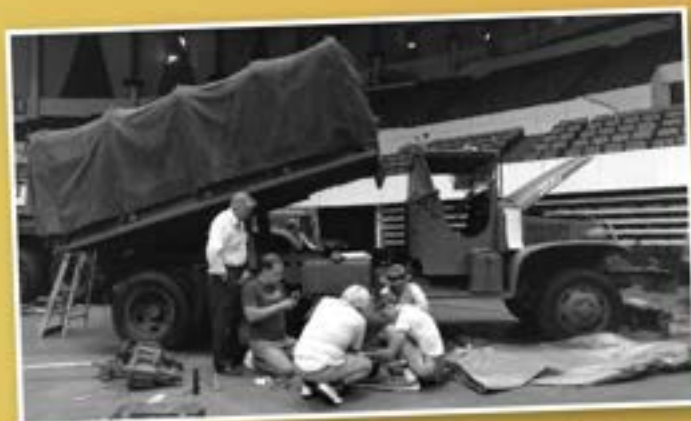
When a GMC CCKW transfer case needed repair at the 1990 Convention in Hampton, Virginia, there were plenty of experts and parts on hand. Jerry Cleveland
