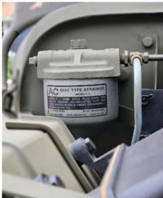
The firewall-mounted AC T-2 fuel strainer was used on WWII jeeps until late 1944.
