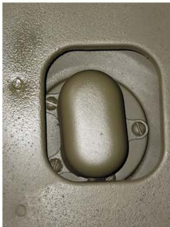
Originally rubber, then changed over to metal, a cover is placed on top of the fuel sender to prevent rubbing or shorting of the top terminal.
