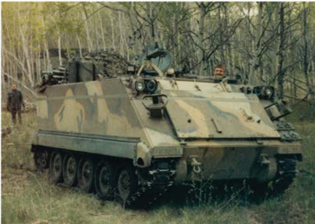
More than 80,000 M113 armored personnel carriers have been produced, making it one of the most widely used armored fighting vehicles in history. Even Canada operated more than 300 from 1964 until 2000. This 62nd Air Defense Regiment M113A1 taking part in RV89 is painted in the MERDC gray desert scheme. W.E. Storey Collection
