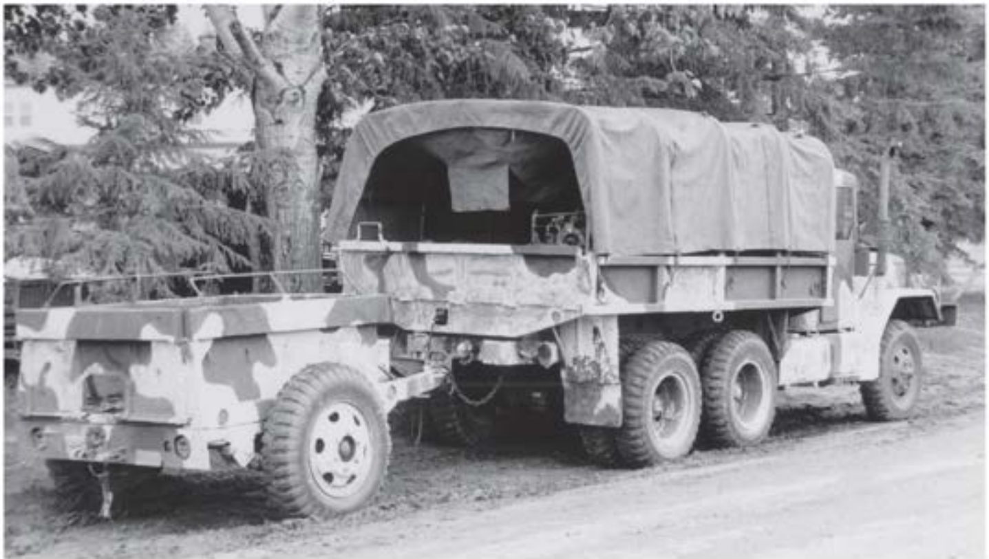
Many of the 172 Brigade vehicles on RV85 were painted in arctic camouflage. This M35A2 2½-ton truck and M332 1½-ton ammunition trailer combination illustrate how the white stood out in Canadian vegetation that consisted of a transitional zone between the grasslands and boreal forest. Mud was used in attempt to cover the white paint. W.E. Storey Collection
