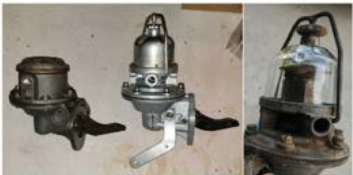
The three most common fuel pumps seen on WWII jeeps have no bowl on top, a metal bowl, or a glass bowl. Only the metal bowl (center) was correct.
