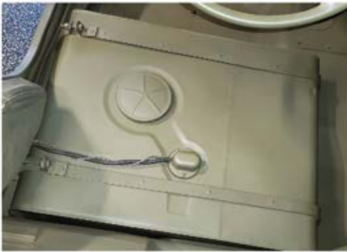
Two straps (made of four parts) were used to strap down the tank to the body tub.
