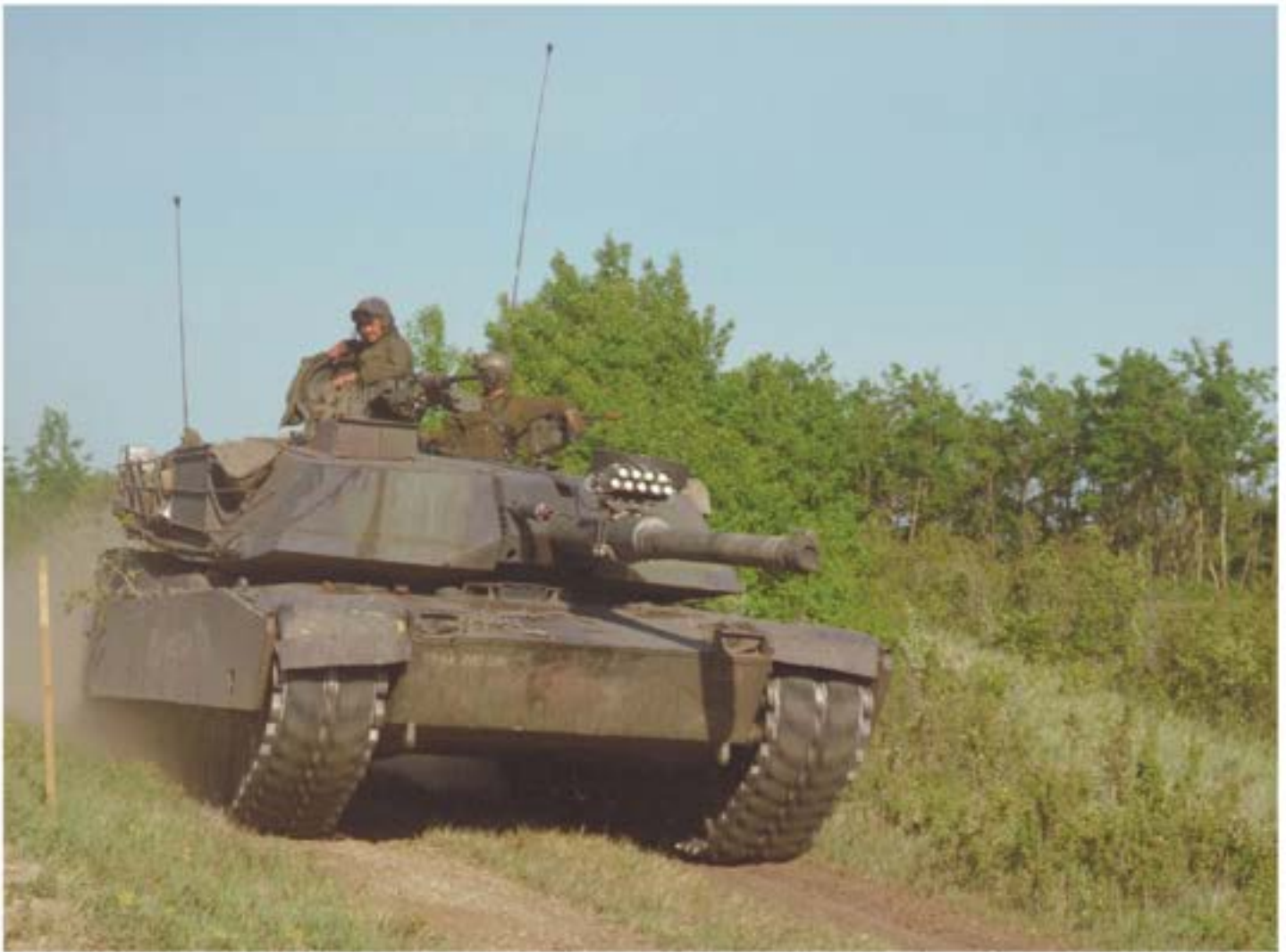
The M1A1 Abrams weighs approximately 67.7 U.S. short tons when fully armed, due in part to its powerful armament and heavy armor – a blend of composite materials like ceramic, metal, and plastic. It has excellent cross-country mobility and speed, with an off-road speed of approximately 25 to 30 mph. This 2nd Battalion, 10th U.S. Cavalry Regiment vehicle from the 194th Armored Brigade was photographed during RV89. Canadian DND CFJIC
