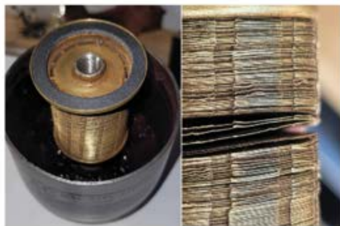
The strainer inside the T-2 was just a compressed stack of brass disks that only allowed fuel to pass between each layer.
