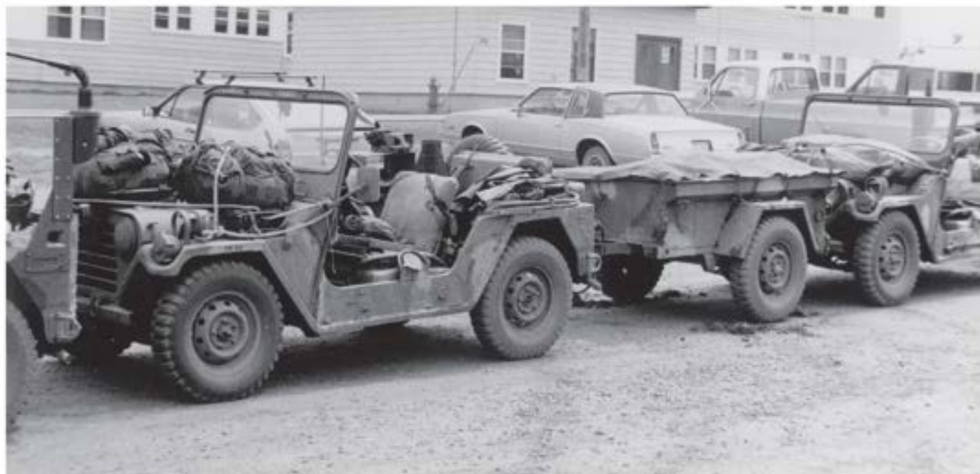
With rucksacks mounted on the front hood and other personal gear slung on the seats or stuffed in the back, these fully loaded RV85 M151A2 MUTTs with their corresponding M416 ¼-ton trailers can provide some inspiration to those who want to correctly stow additional kit on a restored vehicle! W.E. Storey Collection
