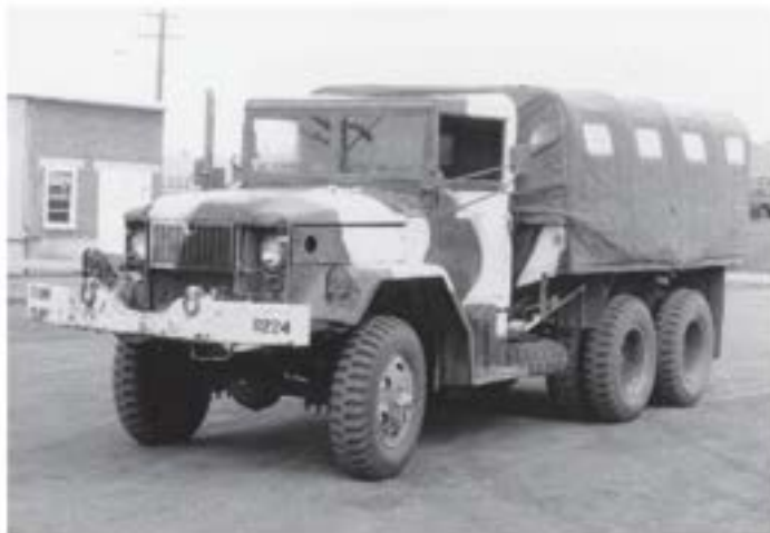
This winter camouflaged 172 Brigade Support Battalion M35A2 2½-ton truck was fitted with a seldom-encountered accessory during RV85: an insulated, cold weather cover for the rear cargo compartment. W.E. Storey Collection
