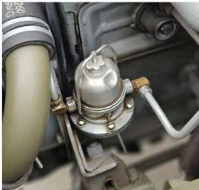
The A.C. fuel pump was located at the lower front driver's side of the engine block.
