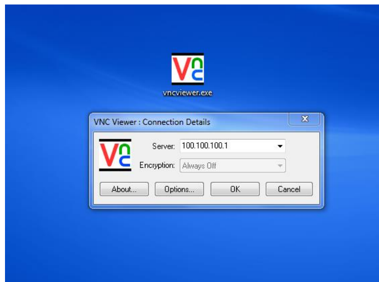
Figure 21: Open a VNC client and introduce smart-G IP address (found in Configuration)
