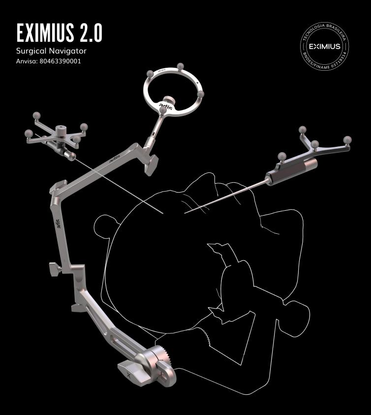
The Eximius Surgical Navigation Image System is indicated for surgeries with a high level of complexity. The navigator provides the surgeon with the real-time spatial location of the instruments in relation to the patient's anatomical and pathological structures on Computed Tomography (CT) and/or Magnetic Resonance (MRI) images.
