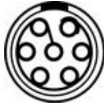
Figure 7: Front face of LEMO 0B 7-pin camera control(single front panel) connector
