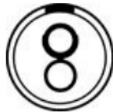
Figure 5: Front face of the LEMO 2-pin power connector
