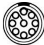
Figure 4: Front face of LEMO 0B 9-pin audio & camera control connector
