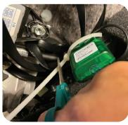
Its always good to trim the excess tie wrap after tightening.
