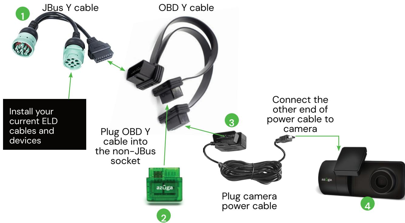
**Note:** some vehicles like Volvo's after 2014 use a 16-pin diagnostics port. If that is the case, you will be supplied with 2 OBD Y cables. Please, use the extra OBD Y cable as you would the Jbus Y Cable in box 1.
