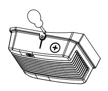
2.Remove the fixing screws and cover plat as shown in Figure 2.
