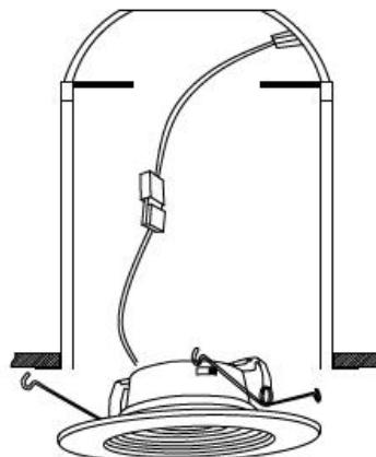
3. Insert the LED Rertofit Kit into the recessed housing unit
