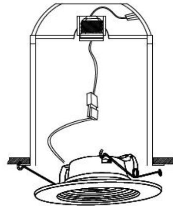
3. Insert the LED Rertofit Kit into the recessed housing unit
