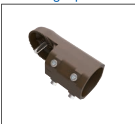
Slipfitter Mount: SZ-AM (03) An optional cast aluminum mast arm adapter secures fixture head to nominal 2-3/8"O.D. horizontal steel tenon arm.
