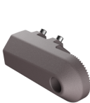
Slipfitter Mount: SZ-AM (500W) (02) An optional cast aluminum mast arm adapter secures fixture head to nominal 2-3/8"O.D. horizontal steel tenon arm.
