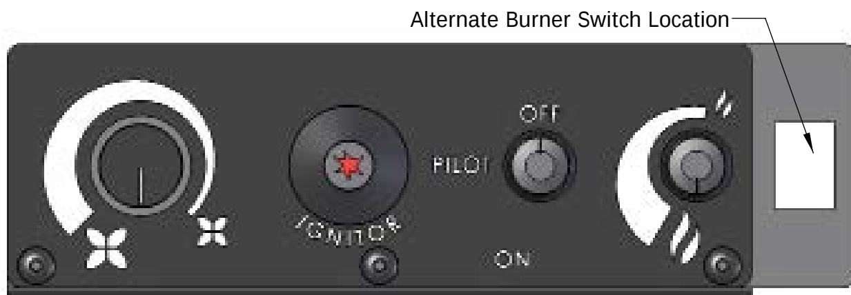
Figure 6: E30 Control Panel.
