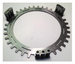
6. Install 0.125" apply plate with slot center over C4 piston orifice.
