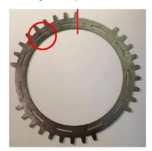
10. Install the C4 backing plate and snap ring.
