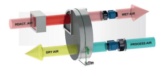
Adsorption dehumidifier technology is based on the use of naturally occurring desiccant materials (i.e. with a high level of chemical/physical affinity with water vapour), such as silica gel.
