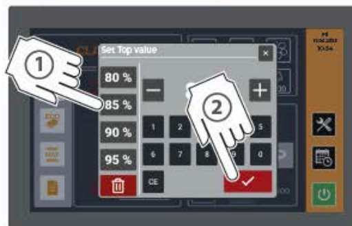
Fig.19 setting top heating element power WITH multiselection
