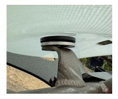
• The stay tabs only have to be parallel to the composite; any gap can be filled with nylon or aluminium spacers without a performance penalty. However, do not use rubber spacers, not only will this allow uncontrolled flexing which will break the edges, but the bolt will be effectively loose, acting like a saw, moving in and out as the seat twists, cutting a slot and allowing the seat to drop.
