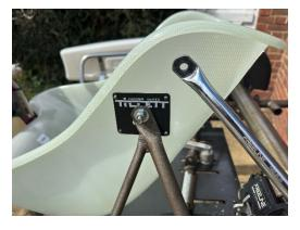
• This will help to adjust the understeer or oversteer on fast corners where the steering wheel is reasonably straight. Move forward if you have understeer and back if you have oversteer. It should be noted that other factors such as width of wheels, chassis/axle/seat flex and steering geometry can affect the handling on tight corners such as a hairpin and can mask this effect.
