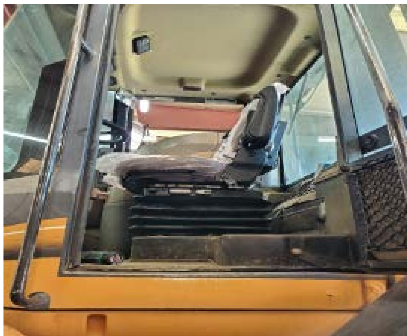
We installed a new seat on loader #5519
