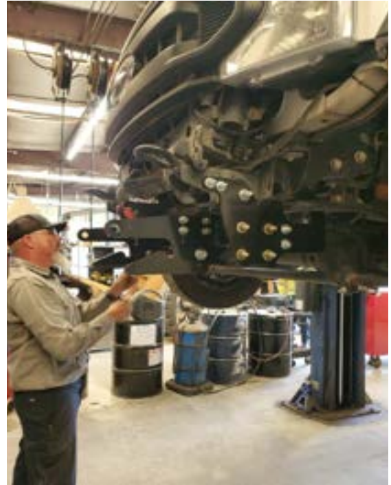
We installed new snowplow brackets under two of the F-550s
