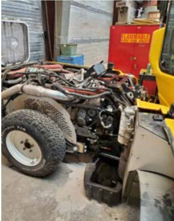
Right of way mower #2209 received a new form-fitted pipe and O rings to fix a hydraulic leak on the hydrostatic motor
