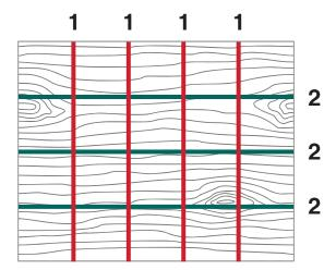
When routing intersecting Dovetail Clamp Tracks, route all cross-grain tracks (1) first, then route the tracks along the grain (2).
