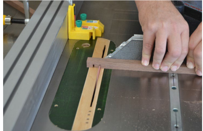
First Half Lap- Leg #3- Fence at 3-5/8"
