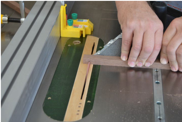
First Half- Lap Leg #1- Fence at 3-5/8"
