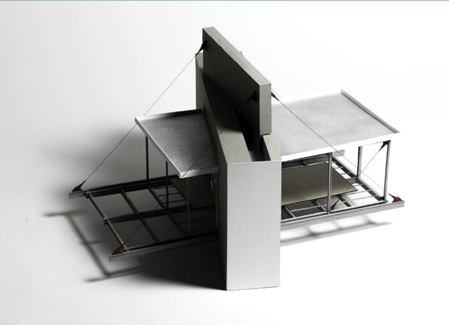
The cantilevering structure highlights the independant nature of the building from the ground that it rests in. Like a T-square, or other scientific tool, it is a framework for controlled reference of environment to study it, and can be removed with little disruption to the existing ecosystem.
