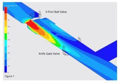
Inlet Pressure: 155 kPa-g Specific Gravity: 1.0 Outlet Pressure: 109 kPa-g Flow: 239 m³/hr
