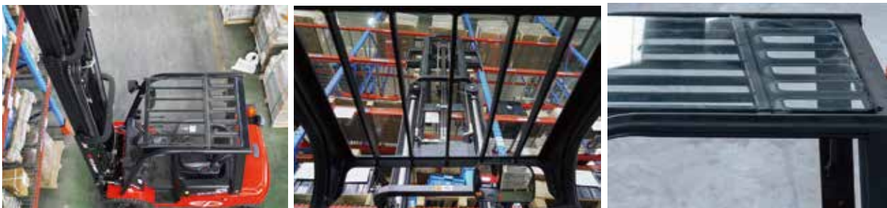
New closed roof
