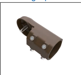
Slipfitter Mount: SZ-AM (03) An optional cast aluminum mast arm adapter secures fixture head to nominal 2-3/8"O.D. horizontal steel tenon arm.
