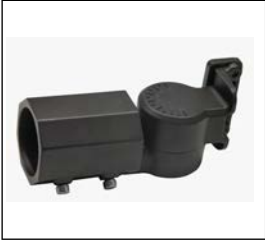
Slipfitter Mount: SZ-AM An optional cast aluminum mast arm adapter secures fixture head to nominal 2-3/8" O.D. horizontal steel tenon arm.
