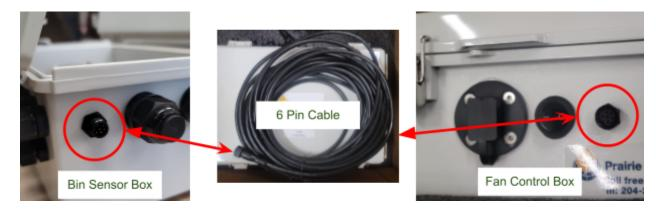
Connect the provided 6 pin cable to the PGA bin sensor box and the fan control box.
