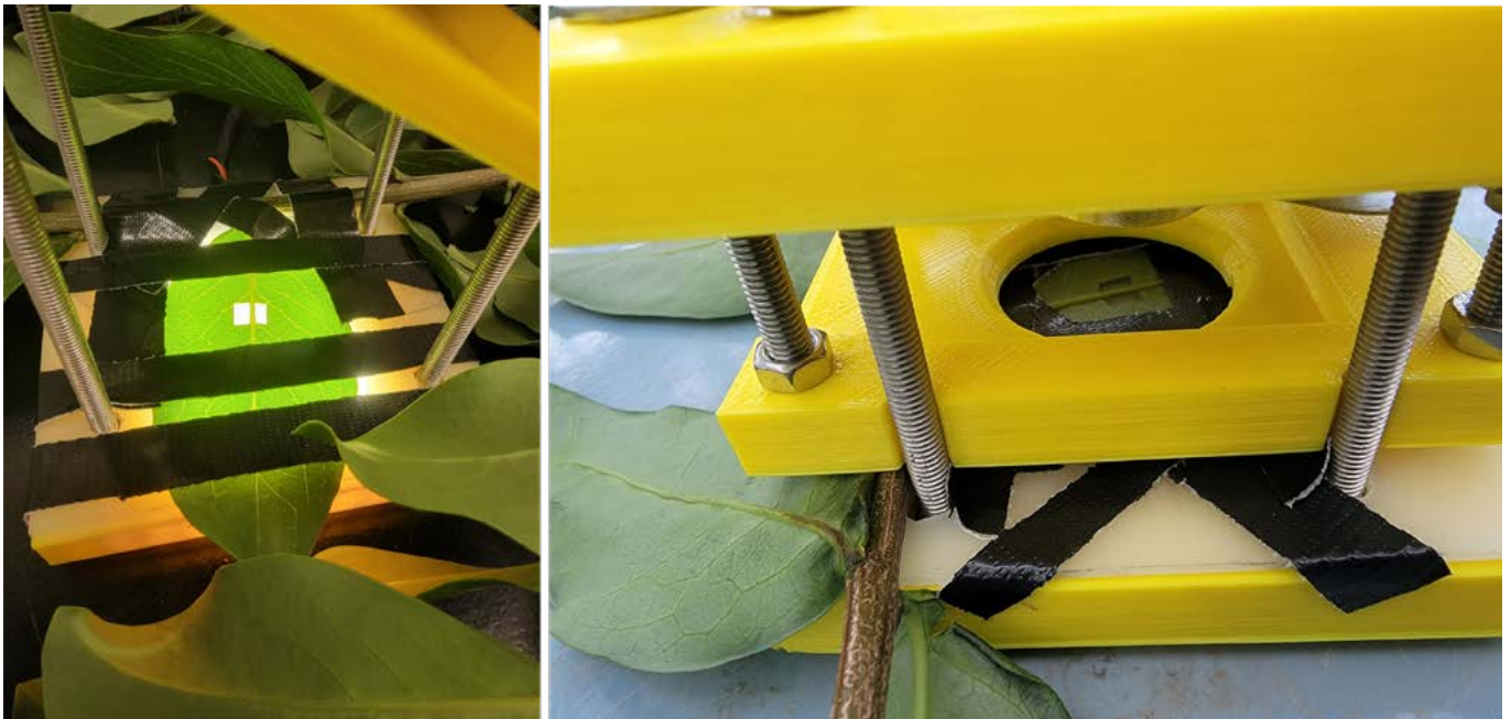
Figure 2: Cavacam set up requires cutting a window of the leaf to create a silhouette of the leaf midrib to detect changes in the leaf midrib area.
