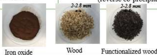
Figure 2. Functionalized woodchip preparation (reverse co-precipitation technique)
