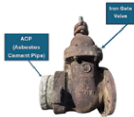
Gate valve cast in 1982, excavated from beneath our roads
