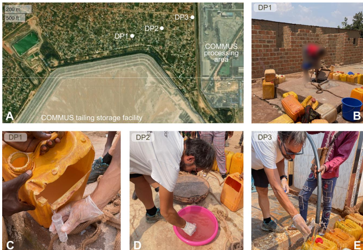
Figure 7. Domestic water sampling in Pierre Muteba II. We sampled 3 domestic water wells near COMMUS’ tailing storage facility and processing area (A), including site DP1 (B-C), DP2 (C), and DP3 (E).
