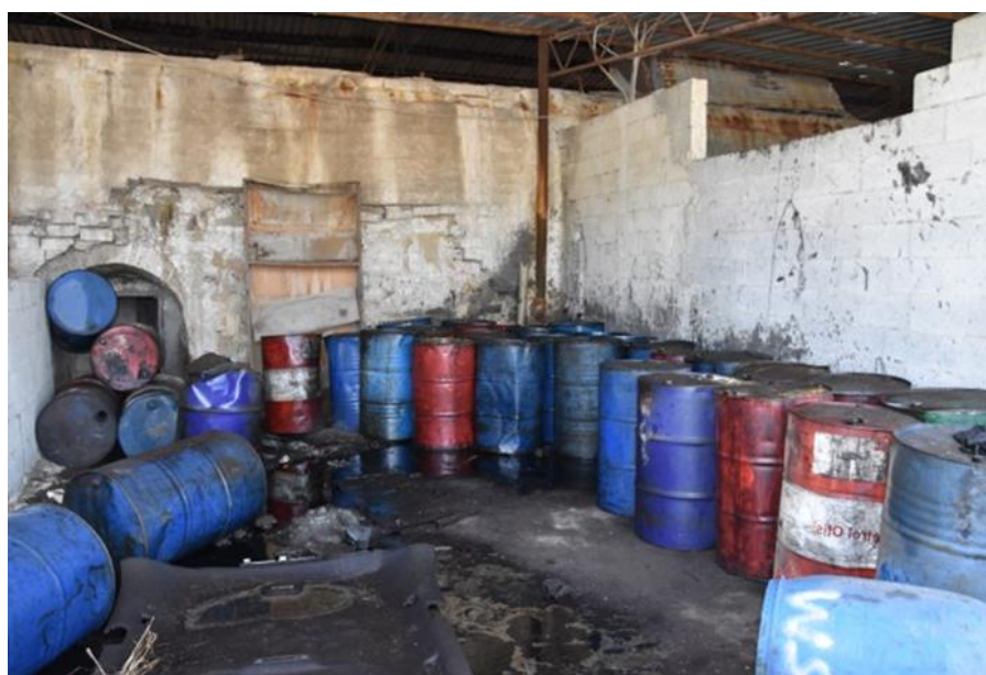
Figure 6. Inadequate storage conditions of chemical drums. Note. Photograph by Huib van Westen.
