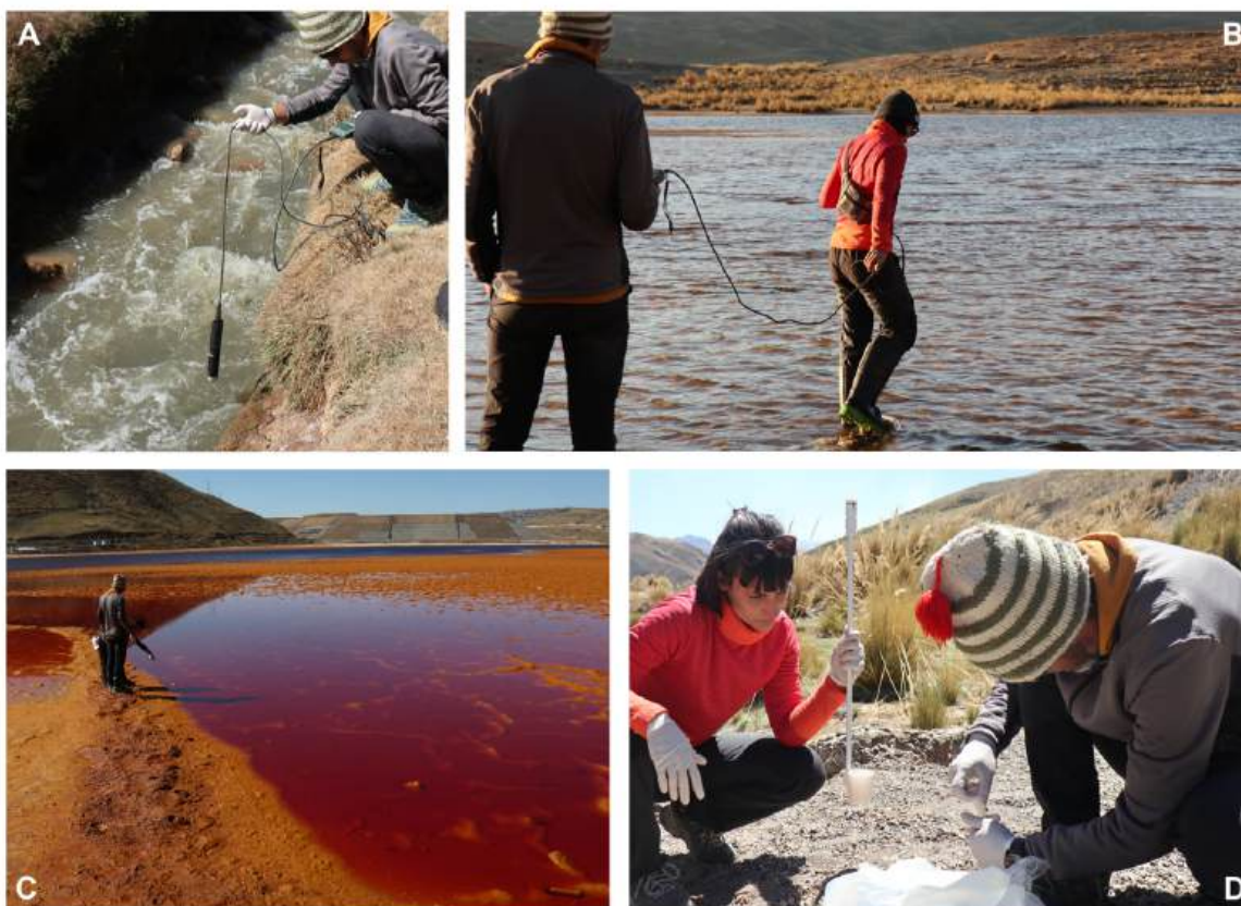
Figure 4. Overview of sampling activities and tools. Panels A and B show the use of the multiparametric probe in the Tingo River and Lake Yanamate. Panels C and D show how we collected surface waters using the Teflon sampler at the Lake Quiulacocha and the Tingo River.
