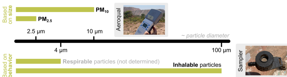
Figure 2. Overview of the parameters monitored in this study. The definition of “PM 2.5 ” and “PM 10 ” (top) is based on particle size, while “respirable” and “inhalable” (bottom) refer to particles’ behavior in the respiratory system – the inhalable fraction get only into the mouth and nose, while the respirable fraction gets deep into the lungs. We measured PM 10 and PM 2.5 with an Aeroqual, while inalable particles were collected with an active sampler and sent to an accredited laboratory for the quantification of heavy metals (more details in the section Sampling and methods ).
