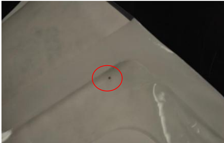
Figure 1: Foreign material located within the accessories pouch
