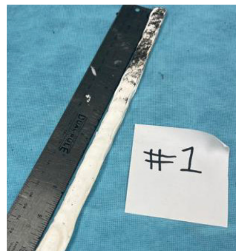
Figure 11 – Sealant #1 recovered to its original length after being bent 180°. Picture taken July 26, 2024.
