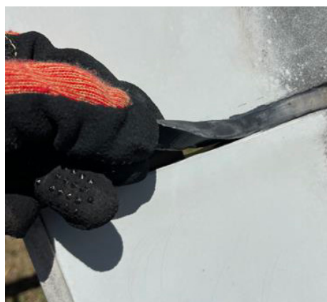
Figure 7 - Sealant #8 was bendable, stretchable, and twistable in the joint. Picture taken April 16, 2024.
