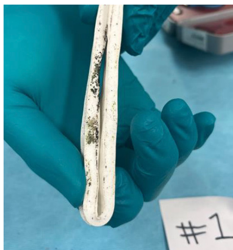
Figure 10 – Sealant #1 bent 180° without any cracking. Picture taken July 26, 2024.
