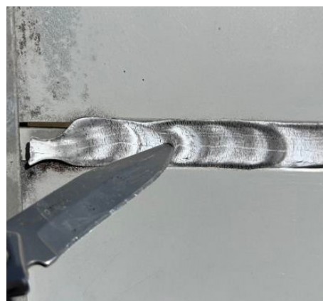
Figure 8 - Sealant #7 resistant to gouging from a pocketknife. Picture taken April 16, 2024.
