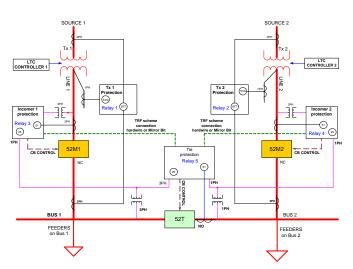
Fig.3 - Main-Tie-Main arrangement with traditionally applied protection and control devices
