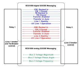
Fig.4 - Digital and analog IEC61850 GOOSE data items exchanged between the two transfer scheme relays
