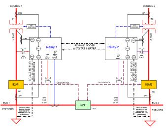
Fig.5 - Main-Tie-Main scheme with two relays performing protection, control and scheme logic
