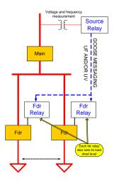
Fig.6 - Load Shed Scheme with GOOSE messaging
