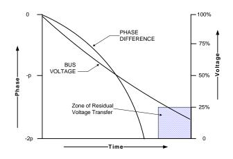
Fig.2 - Voltage decay and phase difference
