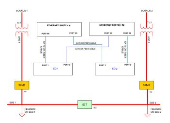
Fig.1 - Main-Tie-Main bus configuration with redundant communication networks
