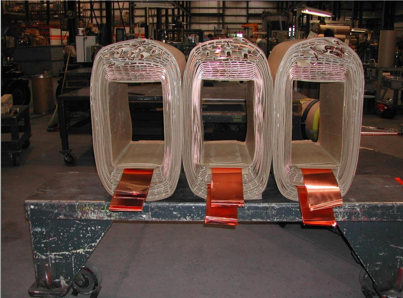
Coils made first then Steel rapped around Coils
