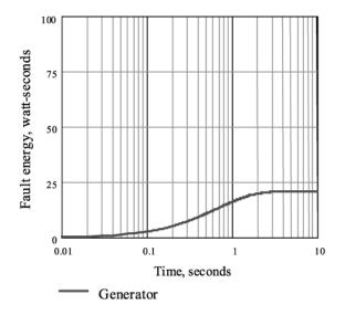
Fig. 9. Fault Energy Versus Time with 10A Grounding
