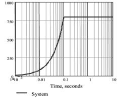
Fig. 7b. Arc Energy due to 400 A "System Current" Over Time
