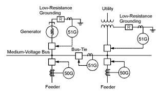
Fig. 21. Generator Ground Time Overcurrent Protection
