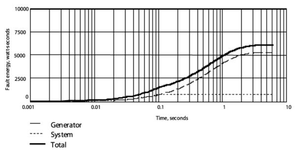
Fig. 10. Fault Energy Accumulation
