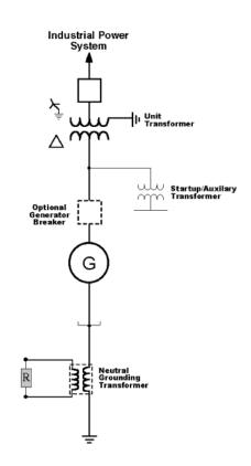
Fig. 11. High-Resistance Grounding of Unit-Connected Generator Configuration
