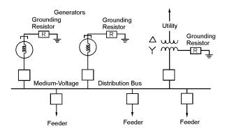
Fig. 1. Medium-Voltage Industrial Distribution System with Multiple Sources
