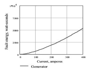
Fig. 8a. Fault Energy due to "Generator Current" – for Various Magnitudes of Current
