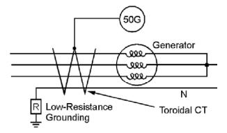
Fig. 22. Instantaneous Ground Overcurrent (Self-Balancing Differential Ground Current) Protection
