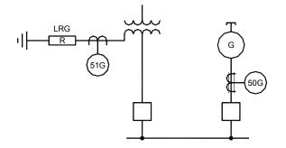
Fig. 15. Generator Ungrounded and System Low-Resistance Grounded
