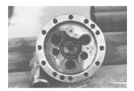
Fig. 14. Failed Motor due to Ground Fault Transient Overvoltage Build-Up
