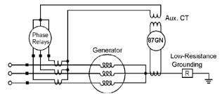
Fig. 20. Generator Ground Differential Protection
