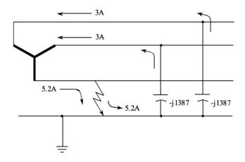
Fig. 12. Ground Faults on Ungrounded Systems
