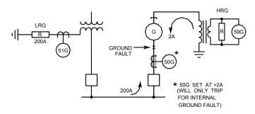
Fig. 16. Generator High-Resistance Grounded and System Low-Resistance Grounded
