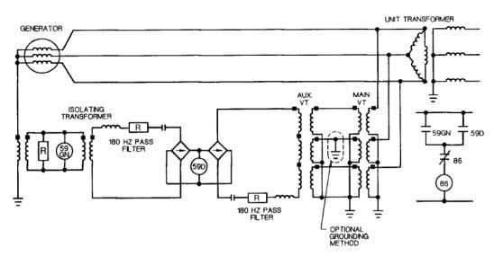
59GN Overvoltage Relay Tuned to the Fundamental (60 Hz) Frequency
