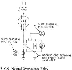
59GN Neutral Overvoltage Relay Tuned to the Fundamental (60Hz) Frequency
