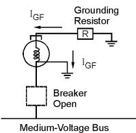
Fig. 2. Generator Internal Ground Fault – Current Flow after Opening Generator Breaker
