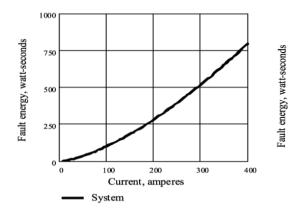
Fig. 7a. Energy due to "System Current – for Various Magnitudes of Current
