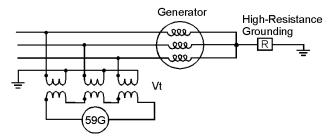
Fig. 23. Wye-Broken-Delta Vt, Ground Overcurrent Protection
