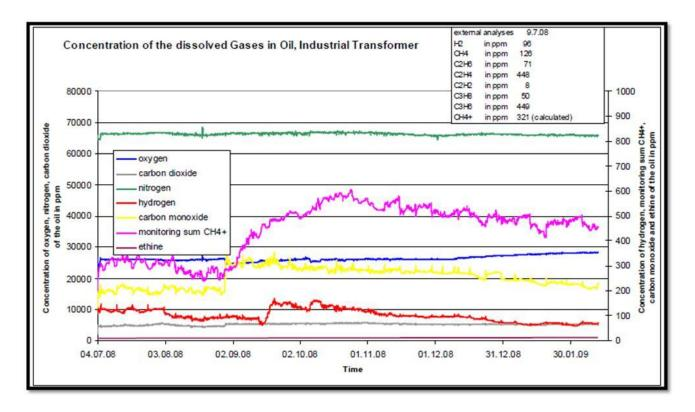
Armed with multiple DGA test data, one can access the need for remedial action. If the test results show continued overheating due to overloading, transferring a portion of the total load to another transformer may be necessary. On the other hand, if a test report reveals the likelihood of internal arcing, a shutdown may be scheduled to allow for an internal inspection of the core/coil assembly to reveal the source.
